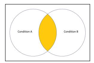
Figure 7: AND Function Diagram
